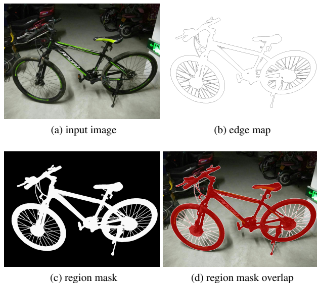
Figure 1. Annotation of a bike. Given an input image, ByLabel computes boundary proposals and the human selects the correct ones. Then, its region mask are generated from these boundaries.
