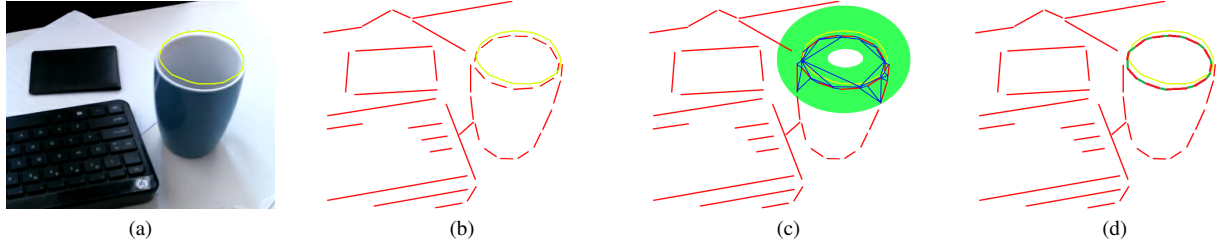
Fig. 2. Illustration of closed boundary tracking: (a) Current image and the tracked boundary ( B_p ) from the last frame (yellow polygon), (b) Detected line segments, (c) Gap filling among line segments in the buffer (green) region of boundary B_p , (d) Tracked boundary ( B_c ) of the current frame.
